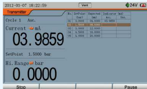
Pressure gauge / transmitter / switch calibration
